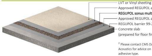
Approved REGUPOL adhesive<sup>2</sup> **REGUPOL sonus multi 530** Approved REGUPOL adhesive<sup>2</sup> REGUPOL barrier 99-201<sup>3</sup> Concrete slab (prepared for floor finishes)
