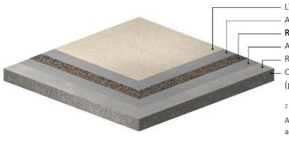
LVT or Vinyl sheeting Approved REGUPOL adhesive<sup>2</sup> **REGUPOL sonus multi 530** Approved REGUPOL adhesive<sup>2</sup> REGUPOL barrier 99-201<sup>3</sup> Concrete slab (prepared for floor finishes)
