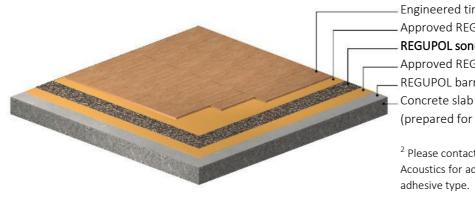
Engineered timber flooring Approved REGUPOL adhesive<sup>2</sup> REGUPOL sonus multi 500 series Approved REGUPOL adhesive<sup>2</sup> REGUPOL barrier 99-201<sup>3</sup>
