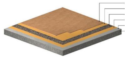
Engineered timber flooring Approved REGUPOL adhesive<sup>2</sup> **REGUPOL sonus eco 3** Approved REGUPOL adhesive<sup>2</sup> REGUPOL barrier 99-201<sup>3</sup> Concrete slab (prepared for floor finishes)
