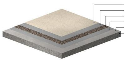
LVT or Vinyl sheeting Approved REGUPOL adhesive<sup>2</sup> **REGUPOL sonus eco 3** Approved REGUPOL adhesive<sup>2</sup> REGUPOL barrier 99-201<sup>3</sup> Concrete slab (prepared for floor finishes)
