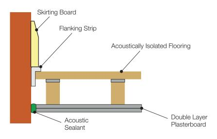
Flanking Strip isolates the flooring system from adjacent structures.
