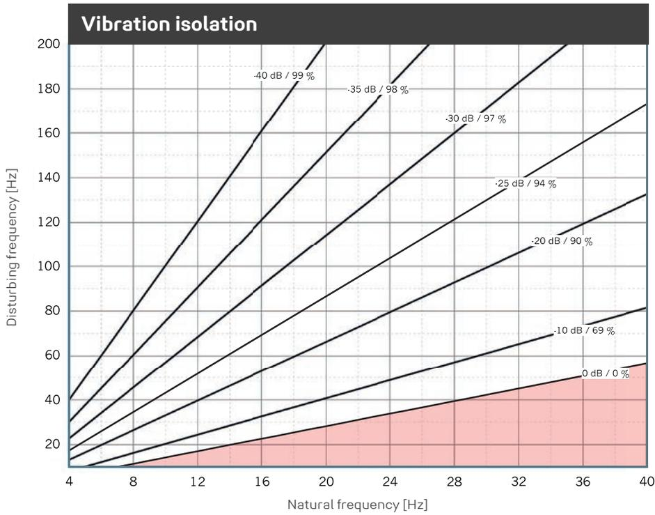
Illustration of the isolation efficiency of a single-degree-of-freedom system (SDOF system) on a rigid base with **REGUPOL vibration 480**. Parameter: power transmission (insertion loss) in dB, isolation factor in %.
