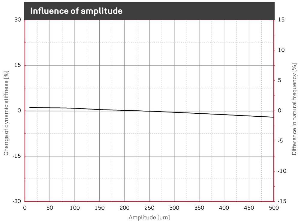
Change of the dynamic stiffness due to changes in amplitudes. Average for 5 Hz, 10 Hz and 40 Hz excitation. Sinusoidal excitation at a constant mean load of 0.600 N/mm<sup>2</sup>, dimensions of the specimens 250 x 250 x 50 mm. Natural frequency of a single-degree-of-freedom system (SDOF system) on a rigid base.
