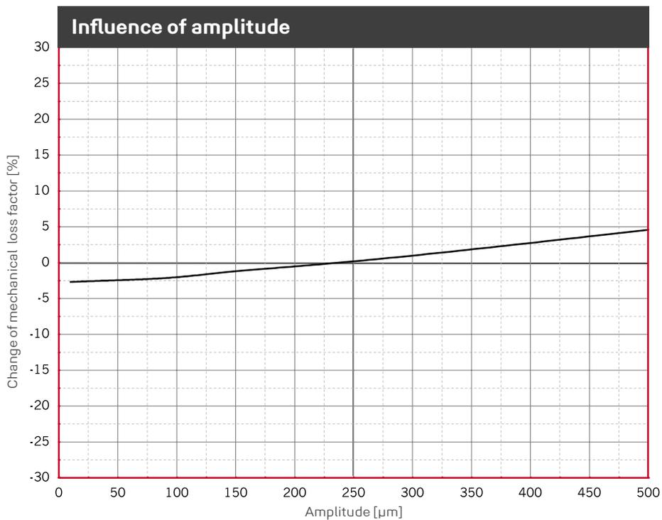
Change of the mechanical loss factor due to changes in amplitudes. Sinusoidal excitation at a constant mean load of 0.600 N/mm<sup>2</sup>, dimensions of the specimens 250 x 250 x 50 mm.
