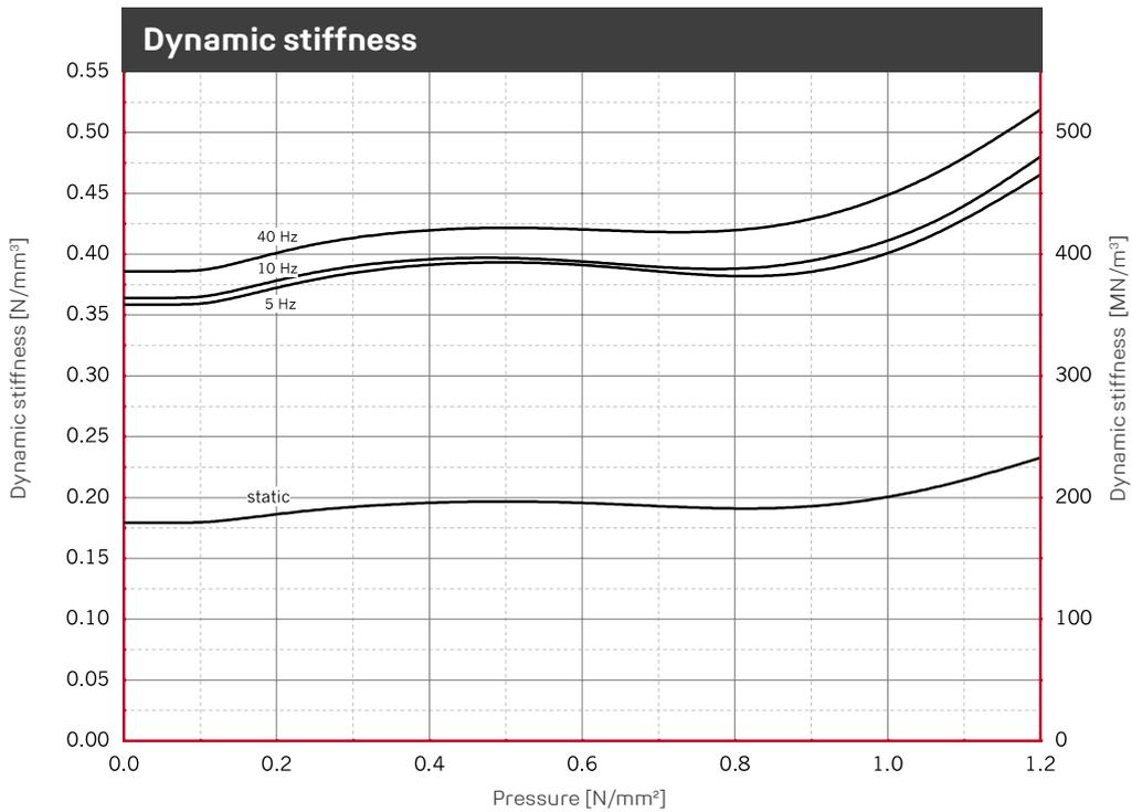
Illustration of the dynamic stiffness for sinusoidal excitation at a constant mean load and an amplitude of  $\pm 0.25$  mm. Dimensions of specimens 250 x 250 x 25 mm; static stiffness as a result of the tangent modulus of the spring characteristic. Tested in accordance with DIN 53513.
