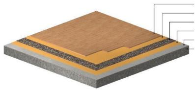
Engineered timber flooring Approved REGUPOL adhesive<sup>2</sup> **REGUPOL sonus multi 4.5** Approved REGUPOL adhesive<sup>2</sup>
