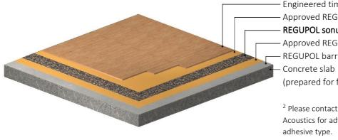
Engineered timber flooring Approved REGUPOL adhesive<sup>2</sup> **REGUPOL** sonus eco Approved REGUPOL adhesive<sup>2</sup> REGUPOL barrier 99-2013 (prepared for floor finishes)
