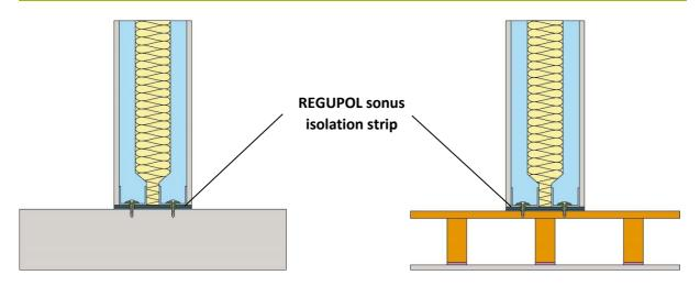
**REGUPOL sonus isolation strips** can be bonded to the applicable subfloor using approved REGUPOL adhesive\* or alternatively, mechanically fix.
