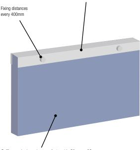
Baffles can be bespoke manufactured in 50mm or 25mm thickness. Typically installed with a 5mm gap between adjacent Baffles
