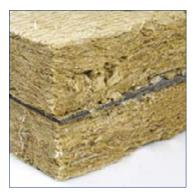
Manufactured from long stranded mineral fibres that are thermo-set with resin into slabs. The inner core of acoustic grade lead or polymeric barrier provides a high degree of resistance to the passage of sound.
