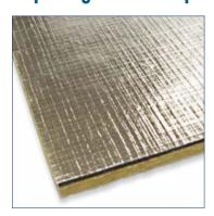
A three-part laminate acoustic insulation for ductwork, pipes and industrial acoustic enclosures. Overcomes the need for a separate isolation layer that is typically required beneath most forms of acoustic lagging.
