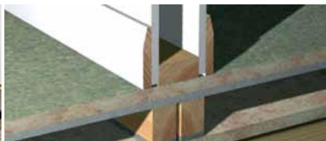
New support of non load bearings partitions
